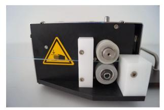
Exactly guidicane for an perfect cut. Fast an easy change of the guidiance, only one screw open.
